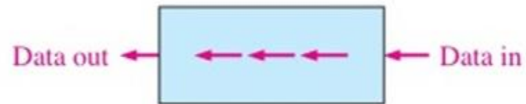
(b) Serial in/shift left/serial out
